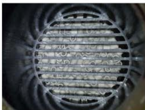
Graphite GT-KELITE grids for 5 tons packing load
