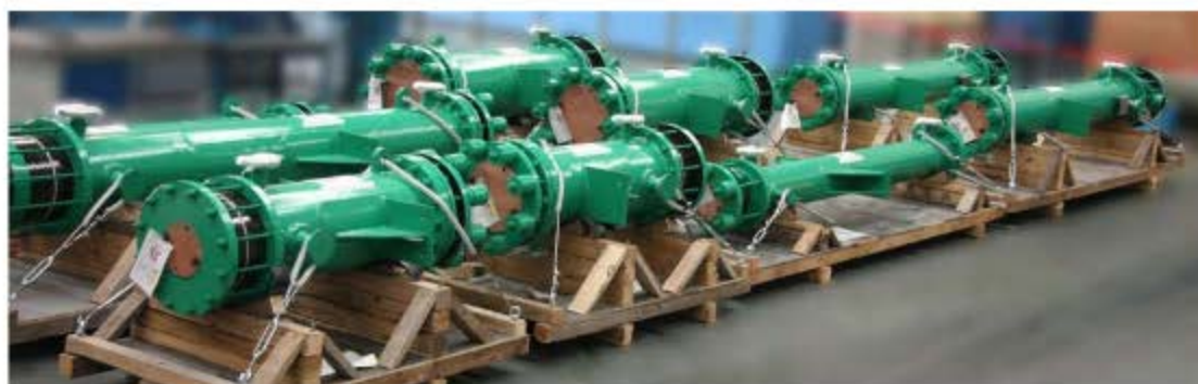
Set of waste gas treatment absorbers in GT KELITE and GT-FLON
